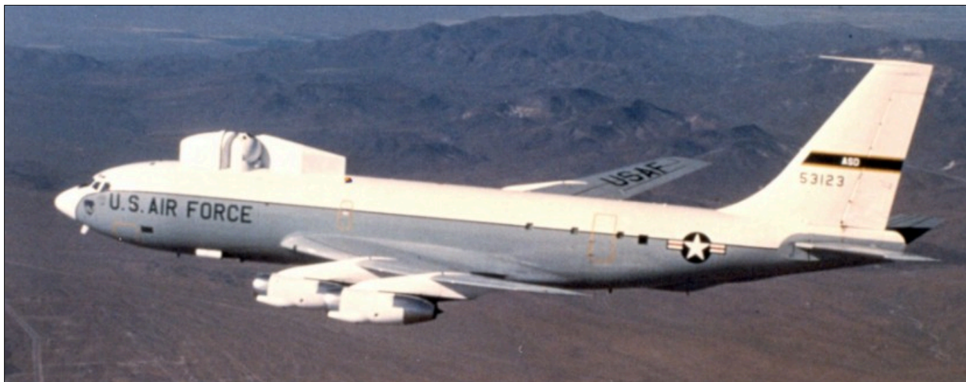
USAF ALL. Note the 60 cm aperture of the telescope. The forward fuselage houses a 10.6 \mu m carbon dioxide gasdynamic laser. The hump aft of the telescope conceals an acquisition and tracking radar system.
