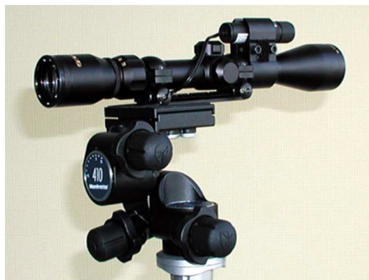
Laser gun sight, zoom rifle scope, 3-axis adjustable tripod head The parts that make this device can be purchased at any gun store and the tripod is a standard issue camera tripod.
