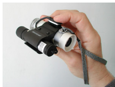
Hand-held unit with laser gun sight and golf scope
